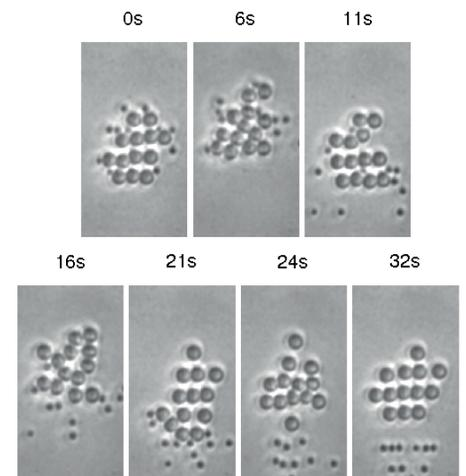
Example of optical sorting of suspension of polystyrene particles of sizes 800 nm and 1600 nm in travelling interference fringes.
