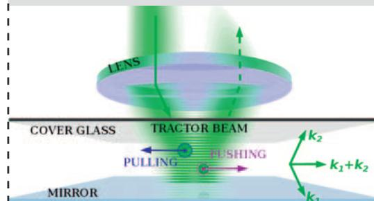
*Geometrical configuration of the tractor beam setup and visualization of the pulling and pushing optical force acting upon particles of different sizes*
