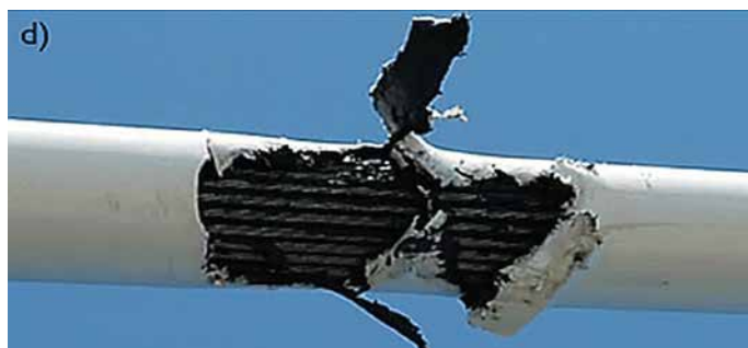
Fig. 1. Examples of icing and rope damage from aeroelastic oscillation.
