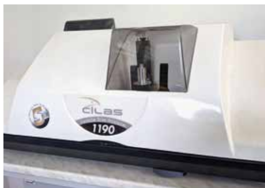
FIG. 10 Cillas 2000 laser particle size analyser in the Geoarchaeology laboratory. Photo by M. Svojtka
