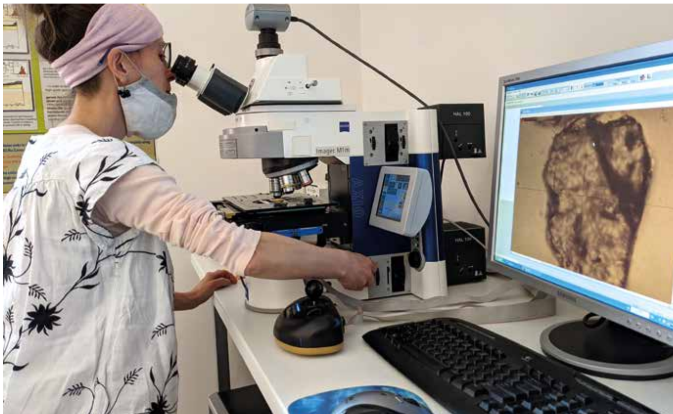
FIG. 7 Fission-track counting system. Photo by M. Svojtka.
