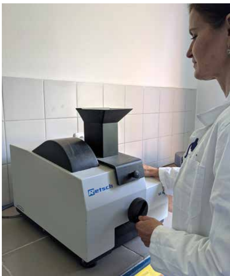
FIG. 6 Dust-tight jaw crusher BB50 Retsch in the separation lab. Photo by M. Svojtka.
