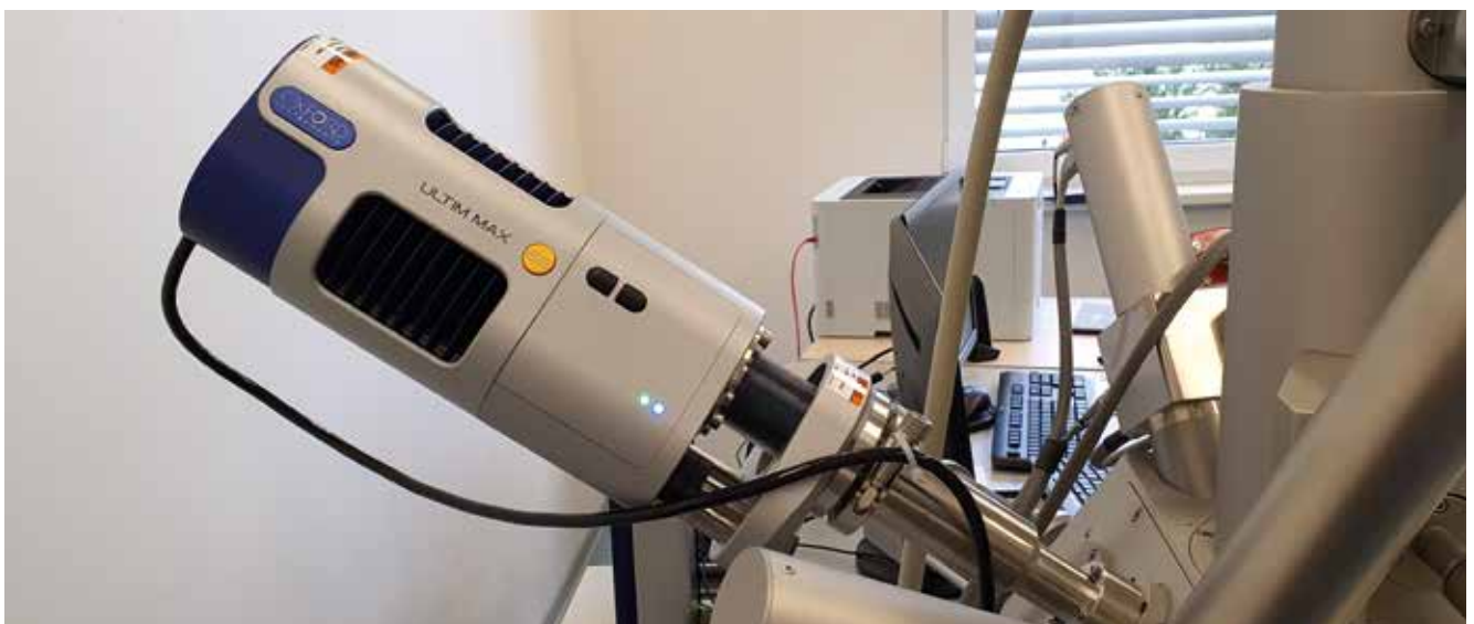
FIG. 4 Energy-dispersive (ED) spectrometer Oxford Ultim Max 65 attached to the scanning electron microscope (SEM) TESCAN VEGA3XMU. Photo by R. Skála.
