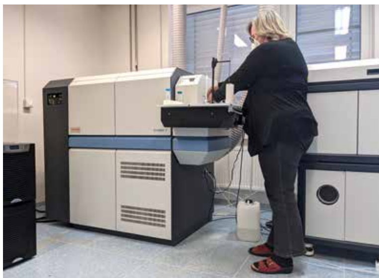
FIG. 8 Laser ablation ICP-MS laboratory with Element2 magnetic sector field ICP-MS and Analyte/Excite excimer 193 nm laser ablation system. Photo by M. Svojtka.
