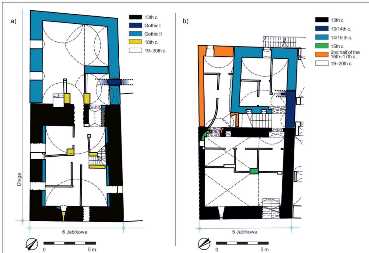
Fig. 75. Brzeg, 5, 6 Jabłkowa Street. Plans of cellars with chronological wall stratification. Preserved walls built in a Vedic way are highlighted in black. After Chorowska et al. 2015, 134, Fig. 3; modified.
