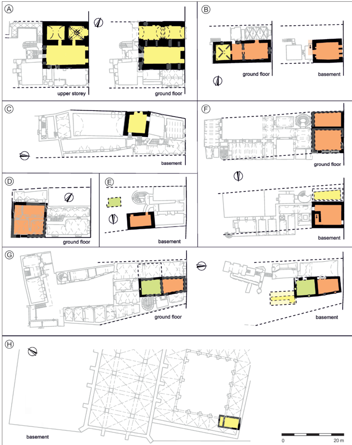
Fig. 112. Selection of layouts and spatial arrangements of Brno's earliest stone houses. Yellow – buildings demonstrably built in the second third of the 13th century; green – after mid-13th century; orange – late 13th and early 14th centuries; A – 8 Radnická Street (Old Town Hall); B – 2 Minoritská Street; C – 7 Zelný trh Square; D – 1 Svobody Square; E – 10 Česká Street; F – 8 Svobody Square; G – 16 Orlí Street; H – Friars Minor friary. Earlier wood-and-clay buildings are also marked with dashed lines for houses E, F and G. Drawing by M. Peška.
