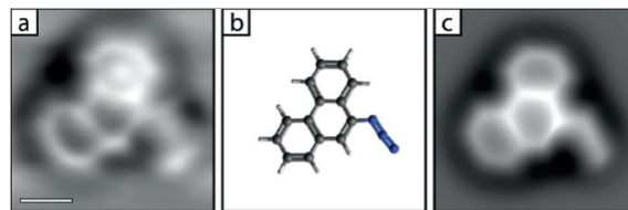
Figure 2. The a) experimental and c) simulated nc-AFM image of the native azide 1 on the Ag(111) surface along with b) the optimised structure of the molecular adsorbate (Ag atoms not plotted for clarity). Scale bar: 500 pm; for a large area experimental image, see Supporting Information, Figure S1.
