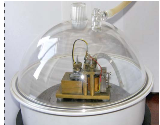
Impact tester in chamber with controlled atmosphere
