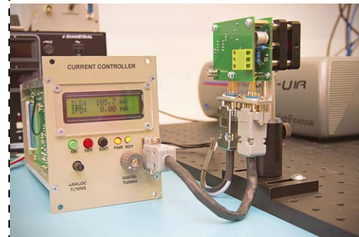
Controller and supporting circuitry for single-frequency laser diode operating in the visible spectral range
