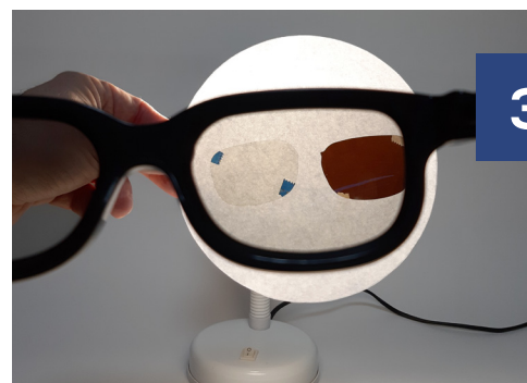
The filters on the paper circle simulate a pair of sunspots of opposite circular polarisation when observed through only one of the filters of another pair of 3D glasses.
