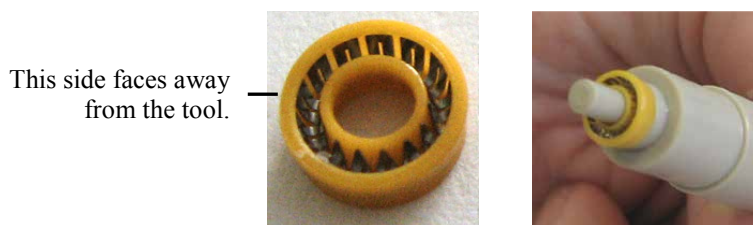
Fig. 72: Correct orientation of the piston seal
