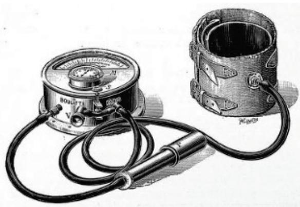
Fig. 8. Original drawing of Pachon oscillometer [53].
