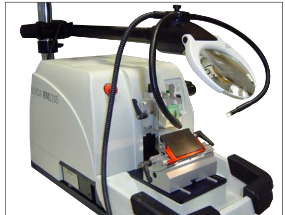
Fig. 71, Leica rotary microtome with installed optional accessories: magnifying lens and fiber-optic light guide
