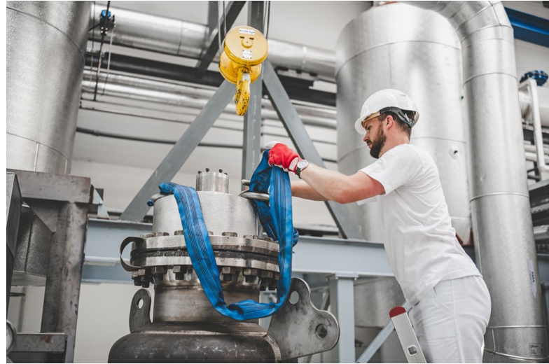
Fig. 4: Manipulation with the cap of the Small LOCA vessel
