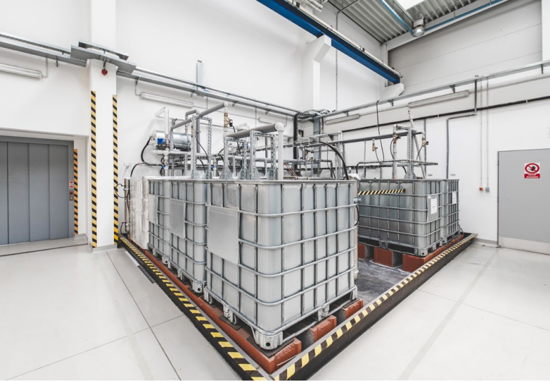
Fig. 3: Water treatment of the LOCA laboratory: vessels with spraying solution and flooding
