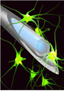
This work has shown for the first time how to unscramble highly disordered images sent down single multimode fibers, making for the narrowest image-guiding system ever. The “order from disorder” approach means that single fibers could be fed down hypodermic needles, sending back deep-tissue images at a range of depths that more complex imaging approaches simply cannot reach.
