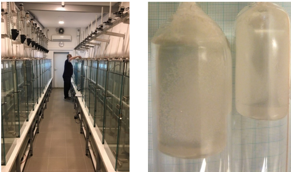
Figure 1. Calomel crystal growth laboratory and finished crystal boules \varnothing 36mm and 28mm.
