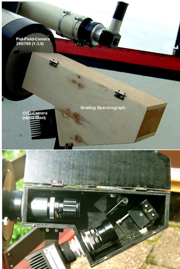
Figure 1: Telescope with spectrograph attached (top) and open instrument (bottom).
