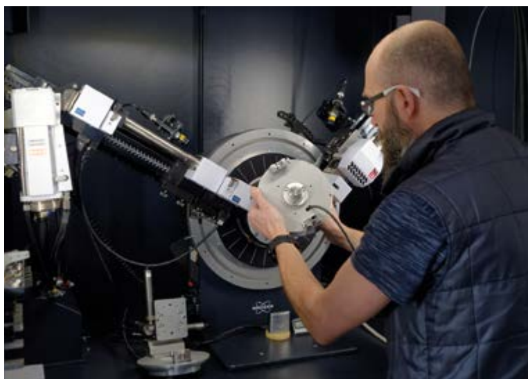
FIG. 13 Placing the corundum calibration standard to the sample holder of the X-ray powder diffractometer Bruker D-8 Discover. Photo by R. Skála.
