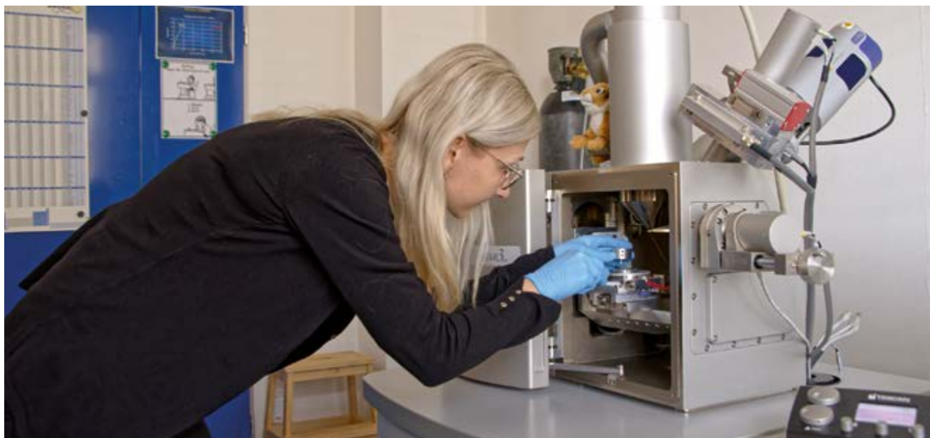
FIG. 6 Inserting the sample to the TESCAN VEGA3XMU scanning electron microscope chamber.
