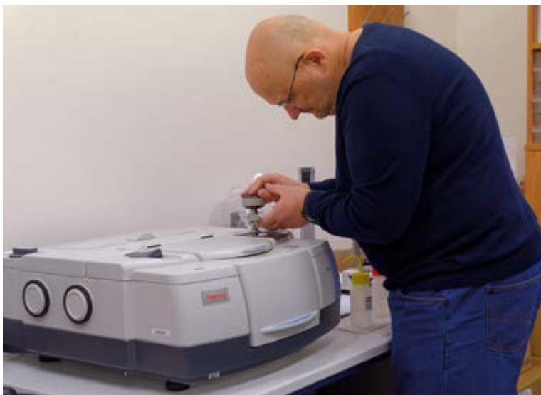
FIG. 11 Acquisition of a Raman spectrum with the microspectrometer Spectroscopy & Imaging Monovista CRS+. Photo by D. Kořínková.
