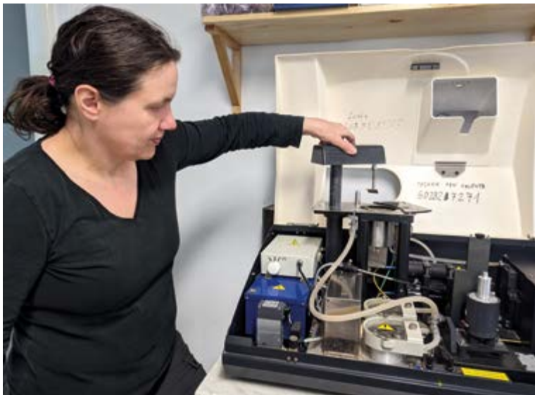
FIG. 3 Sample preparation on the Cilas 1190 laser particle size analyser in the Geoarchaeology lab. Photo by M. Svojtka.
