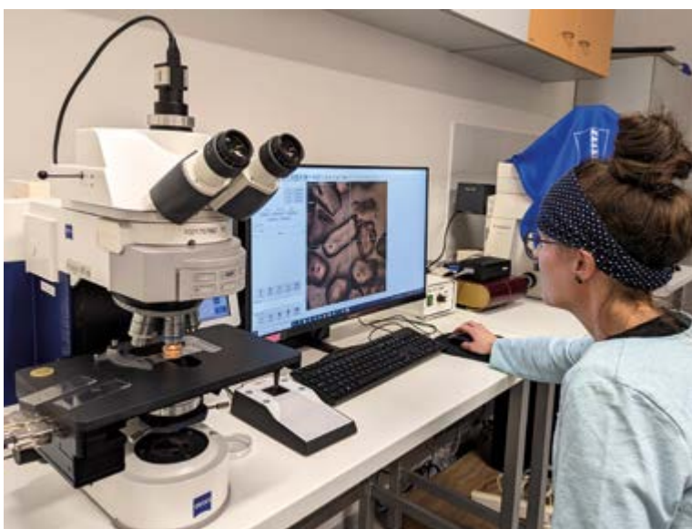
FIG. 2 Automated Zeiss microscope counting system in the Fission-track lab. Photo by M. Svojtka.
