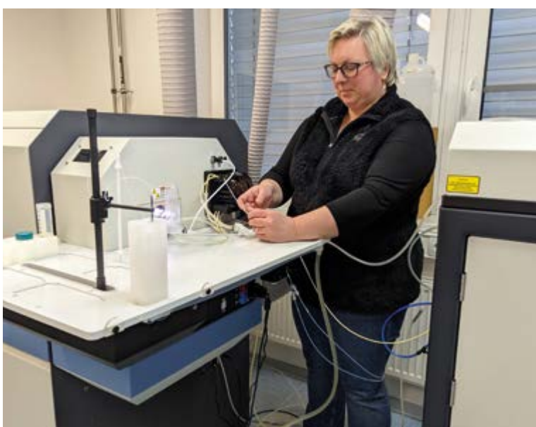
FIG. 5 Sample introduction system, which is a part of high-resolution Element 2 magnetic sector field ICP-MS (left) connected with a Analyte/Excite excimer 193 nm laser ablation system (right) in the ICP-MS lab. Photo by M. Svojtka.
