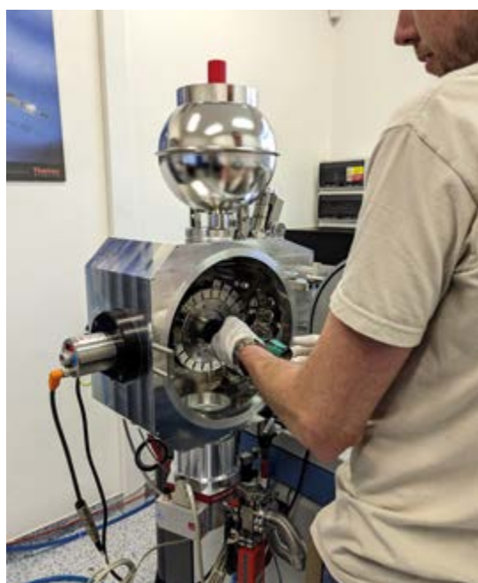
FIG. 17 The exchange of the sample turret in the ion source housing of the Triton Plus instrument in the TIMS lab. Photo by M. Svojtka.
