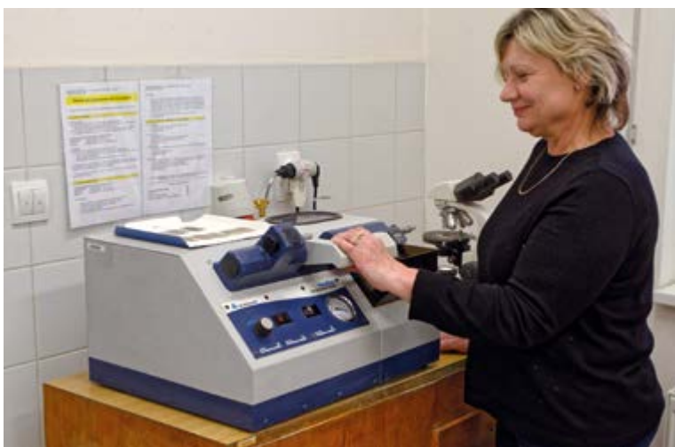
FIG. 4 The Buehler PetroThin is a precise thin section cutting machine for re-sectioning and thinning of rock, mineral, and other solid-state samples. Photo by R. Skála.
