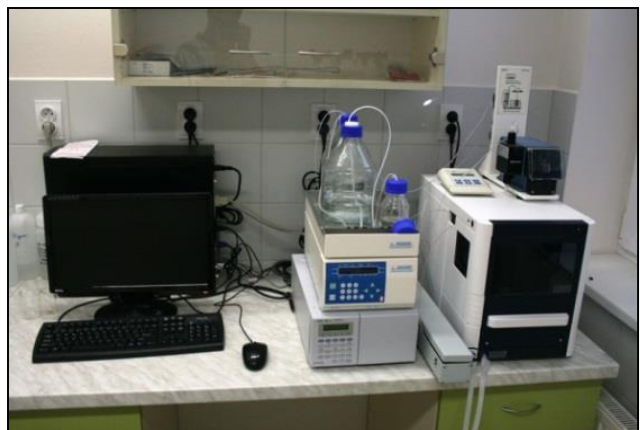
The presence and amount of nitrates, chlorides, sulfates and other anionic component is analysed on the HPLC liquid analyser by chromatography on anion exchanging chromatography with conductivity detection.
