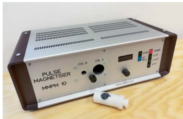
■ Fig. 3. A new Magnetic Measurements MMPM10 Pulse Magnetizer. Photo by T. Elbra.
