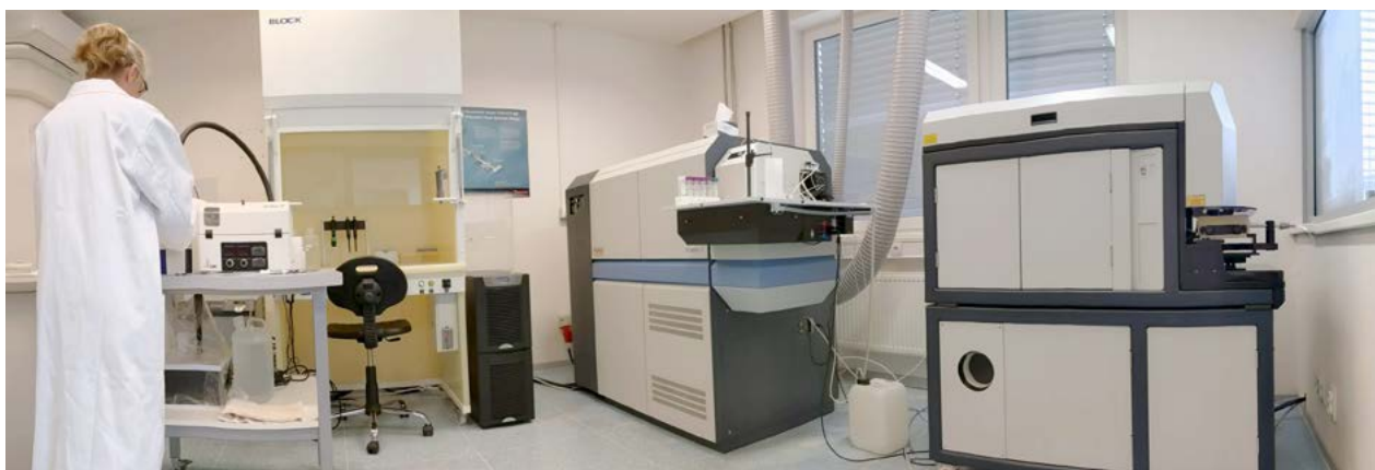
■ Fig. 6. Laser ablation ICP-MS Laboratory. Photo by M. Svojtka.
