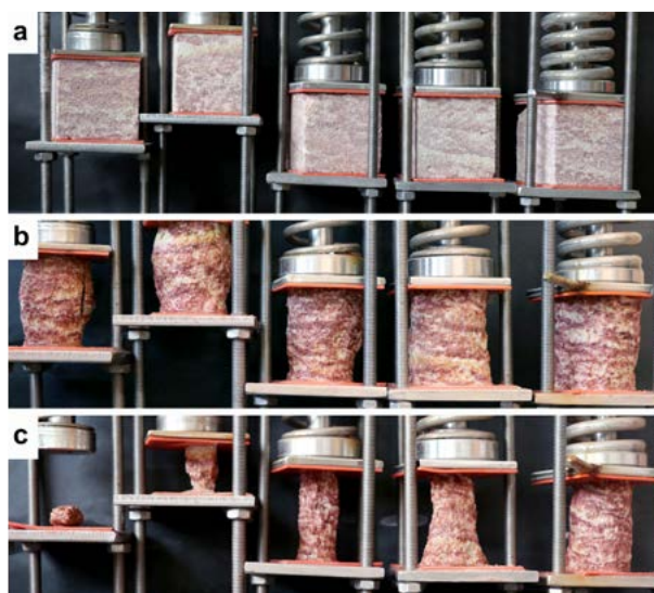
■ Fig. 27. One of the freezing/melting experiments with differently loaded Střeleč sandstone cubes: a) initial state, b) after 10 cycles, c) after 60 cycles. Loading of cubes from left: 30N, 65N, 122N, 240N, 480N. The experiment clearly shows that higher loading reduces the erosion. Photo by M. Filippi.
