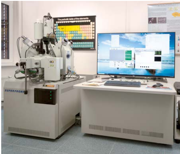
■ Fig. 2. Electron microprobe analyzer JEOL JXA-8230 installed at the Laboratory of Electron Microanalysis in November 2019. Photo by R. Skála.
