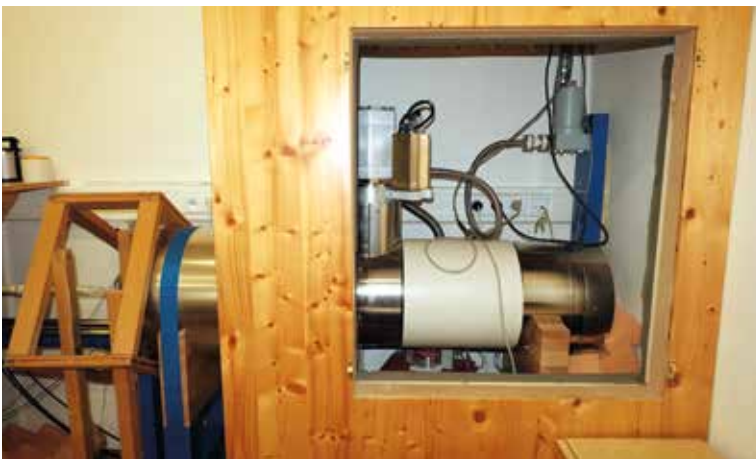
FIG. 9 2G 755 4K Superconducting Rock Magnetometer. Photo by J. Petráček.
