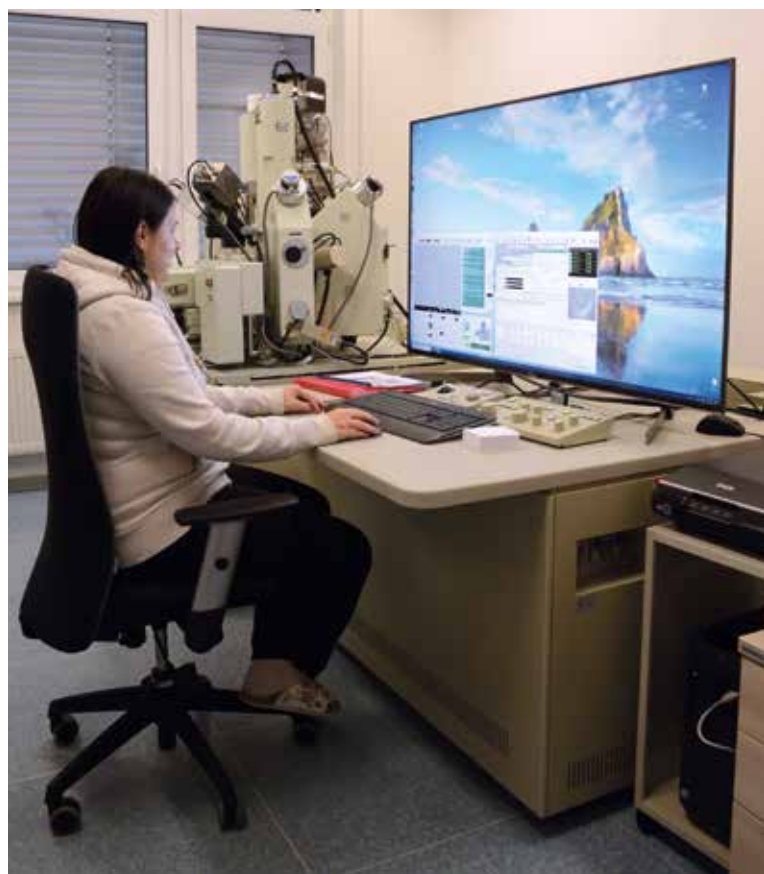
FIG. 6 Taking analysis with the electron probe microanalyzer JEOL JXA-8230. Photo by R. Skála.
