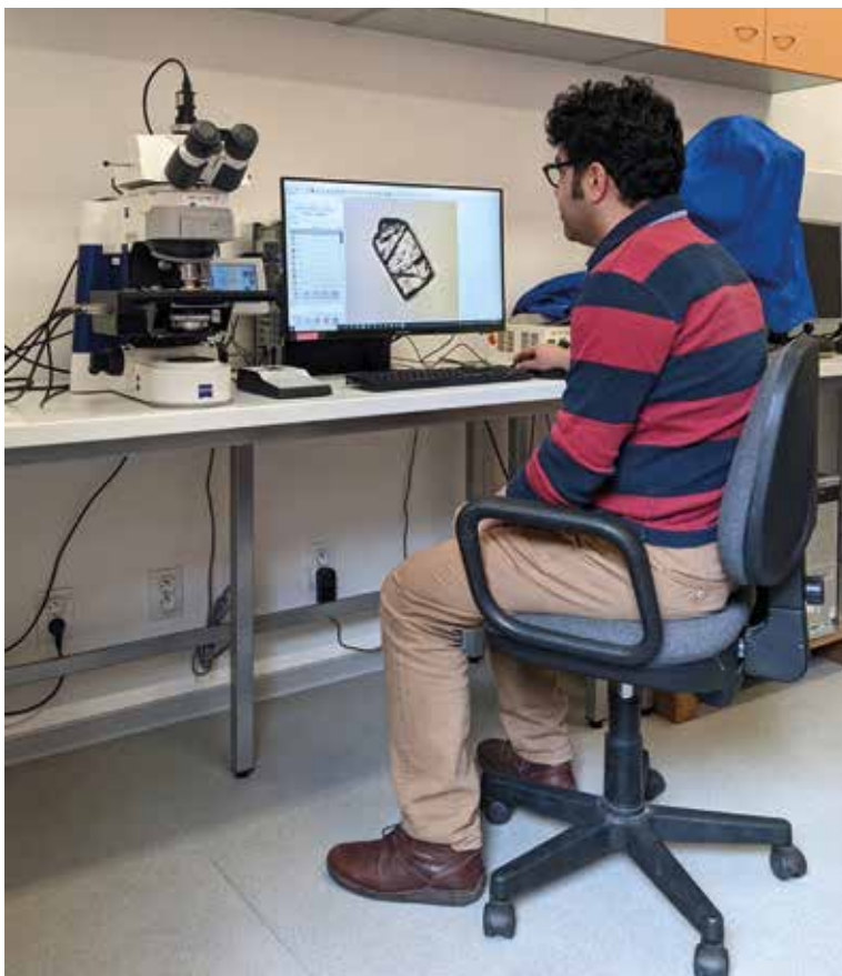
FIG. 2 Fission-track counting system. Photo by M. Svojtka.
