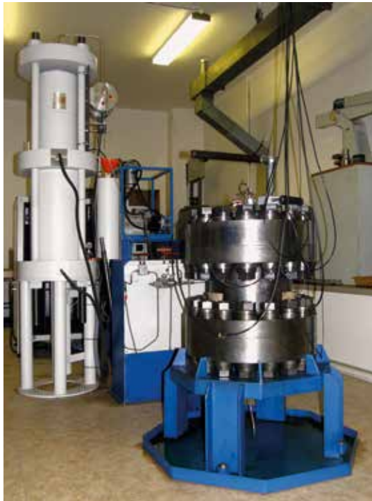
FIG. 10 Hydrostatic pressure vessel for measurement of detail, P and S wave, velocity anisotropy. Photo by V. Filler.
