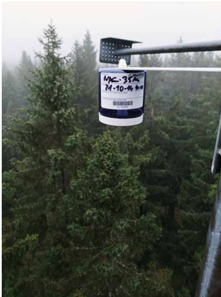
FIG. 35 Exposed passive sampler for monitoring atmospheric mercury 35 m above the ground at the top of a monitoring tower, Načetín experimental site. Photo by T. Navrátil.
