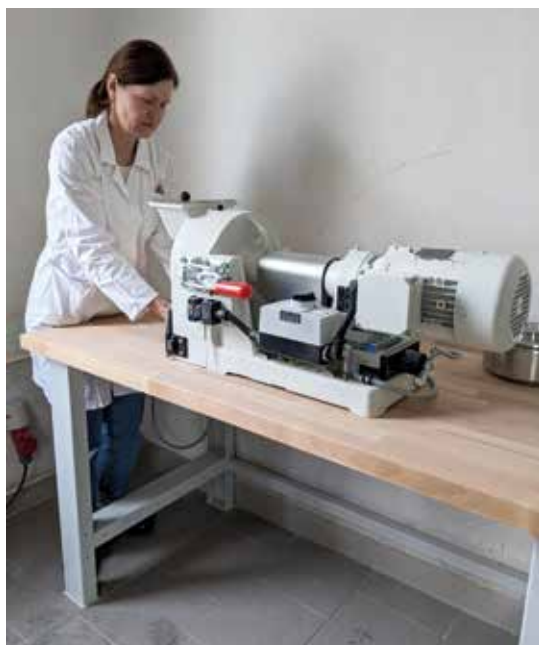
FIG. 12 A new disk mill Pulverisette 13 (Fritsch) was acquired in the Mineral Separation Lab. Photo by M. Svojtka.
