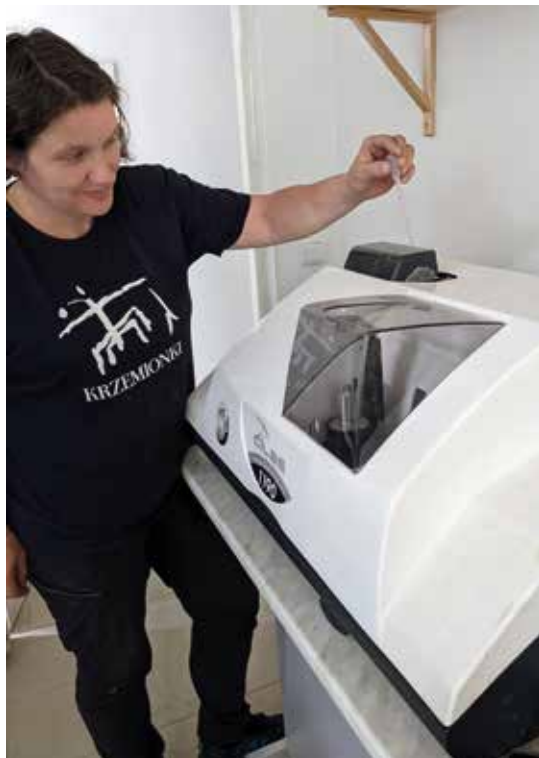
FIG. 3 Cilas 1190 laser particle size analyzer in the Geoarchaeology Laboratory. Photo by M. Svojtka.
