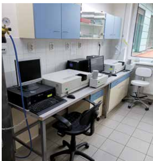
FIG. 14 A pair of cold vapor atomic absorption spectrometers AMA-254 by Altec, Prague with autosamplers and power backup station. Photo by T. Navrátil.
