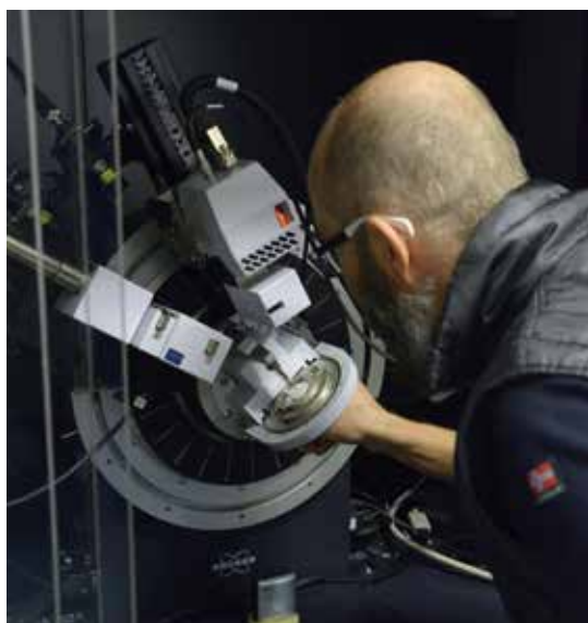
FIG. 13 Placing the corundum calibration standard to the sample holder of the X-ray powder diffractometer Bruker D-8 Discover. Photo by R. Skála.
