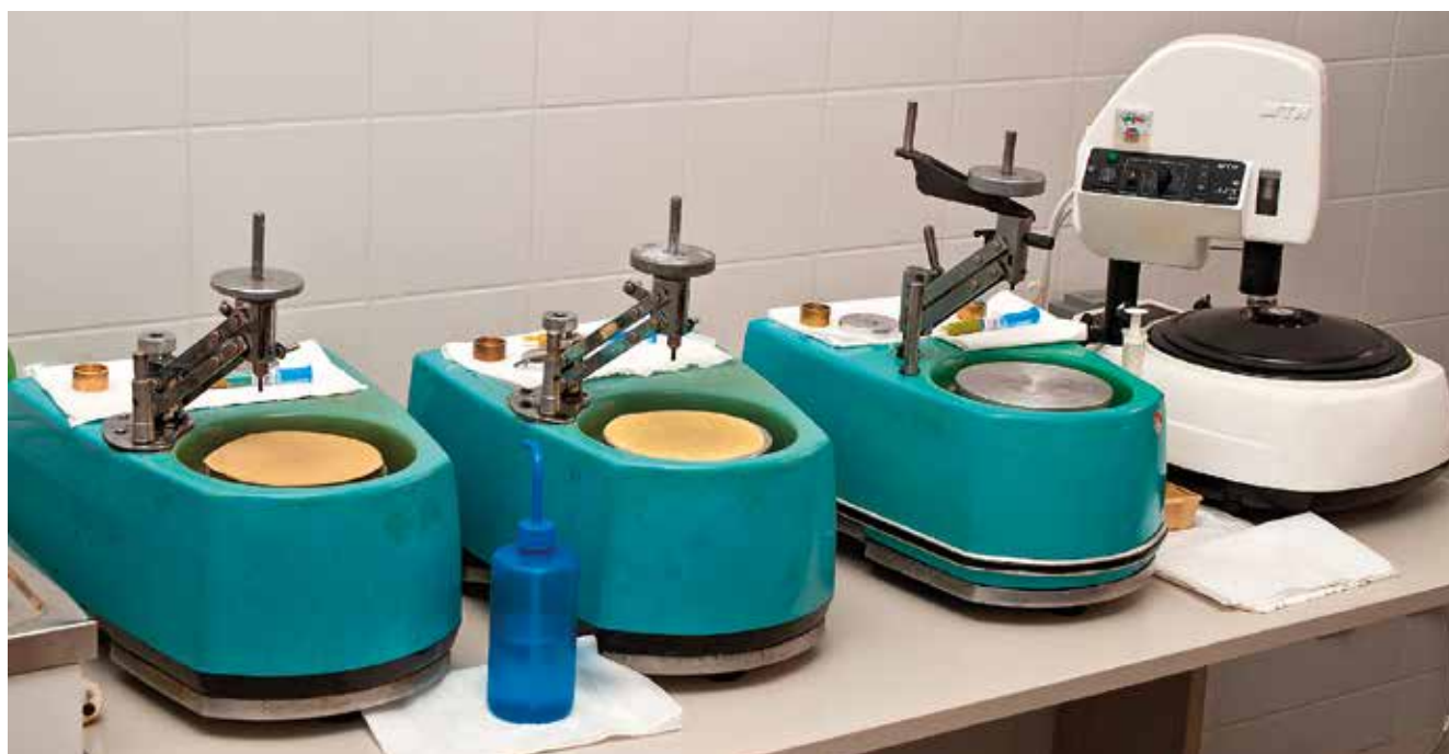
FIG. 4 Grinding machines with diamond plated wheel Montasupal and custom-made grinding machines with wheels for loose abrasive powder. Photo by R. Skála.
