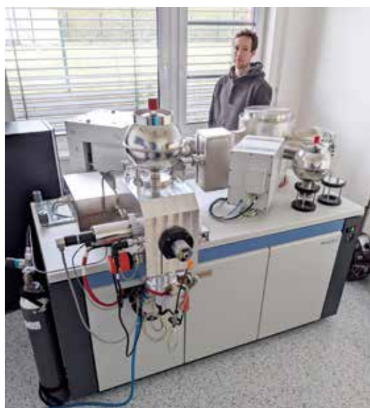
FIG. 17 Triton Plus mass spectrometer (TIMS laboratory). Photo by M. Svojtka.
