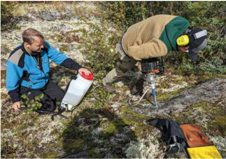
FIG. 26 Field sampling for the anisotropy of magnetic susceptibility (AMS) analysis. The studied rocks are porphyritic monzonites of the Radisson Pluton and the drilling of the samples is carried out by L. Ackerman and F. Tomek. Photo by M. Svojtka.
