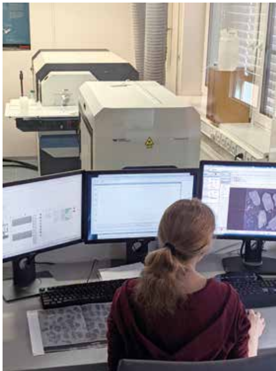
FIG. 5 Laser ablation ICP-MS laboratory with Element2 magnetic sector field ICP-MS and Analyte/Excite excimer 193 nm laser ablation system. Photo by M. Svojtka.
