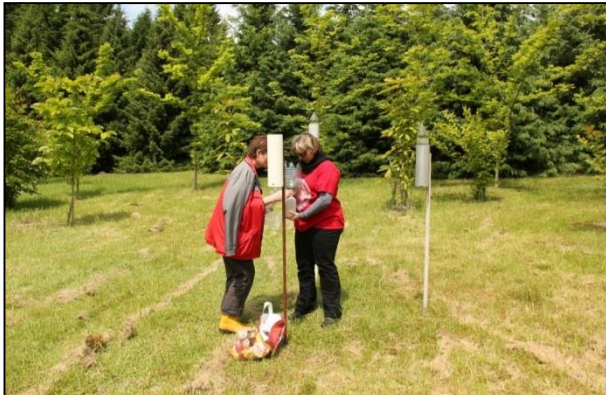
Collection of an environmental sample: Passive collector for collection of rain water.
