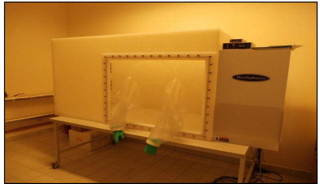
Glove-box where inside the closed space, argon atmosphere is maintained to protect the sample from air influence and contamination from atmospheric dust. Samples are inserted by the port to the right site and handled by gloves connected to long plastic sleeves.
