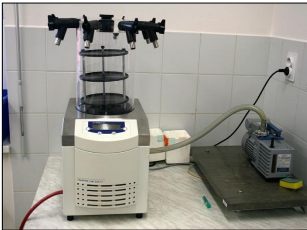
The freeze-drying apparatus is frequently used in biochemical and biological applications for careful drying of sensitive samples. Samples are frozen before drying in vacuo , water is removed from the sample by sublimation.
