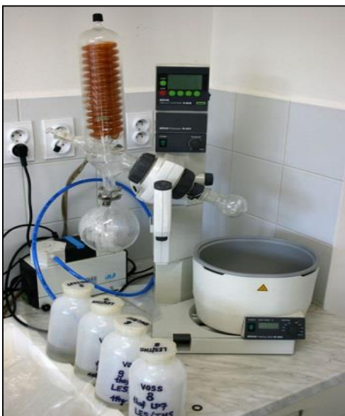
Diluted liquid samples can be preconcentrated before analysis on the vacuum rotary evaporator . Samples are delivered in the plastic bottles, transferred into an evaporation flask and evaporated in vacuo . Concentrated sample resulting is present in a small flask connected to the apparatus.
