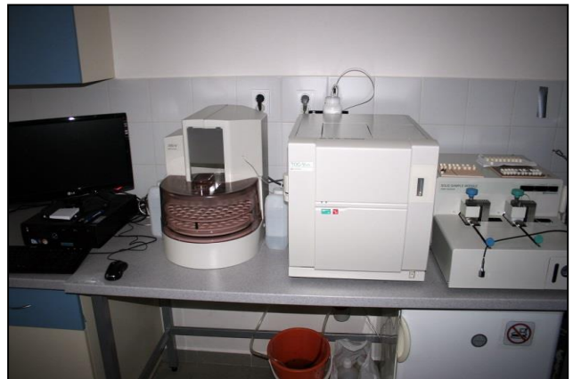
Quantification of inorganic carbon (carbonate) and organic carbon in natural liquid or solid samples is performed on TOC analyser equipped with autosampler for liquid samples introduction.
