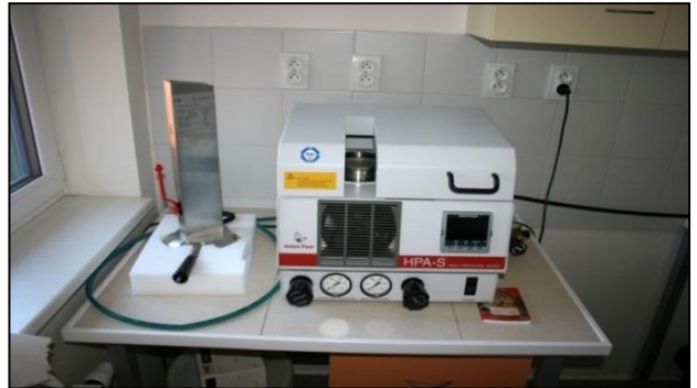
Before analysis, majority of solid samples are prepared by decomposition in acids. In the HPA-S Anton Paar high pressure asher , samples are dissolved at temperatures up to 300 °C and pressures up to 100 atm.
