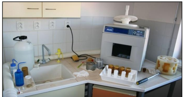
Microwave oven is not only useful in a house kitchen, but with a special teflon PTFE pressure vessels it is equally useful for sample decomposition. Of course, the microwave power inserted on sample is far more higher than in the kitchen models.
