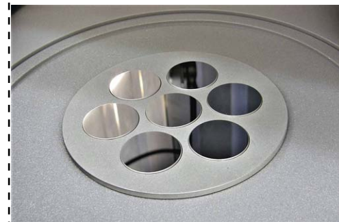
Example of an Ag-based laser mirror on a glass substrate.
