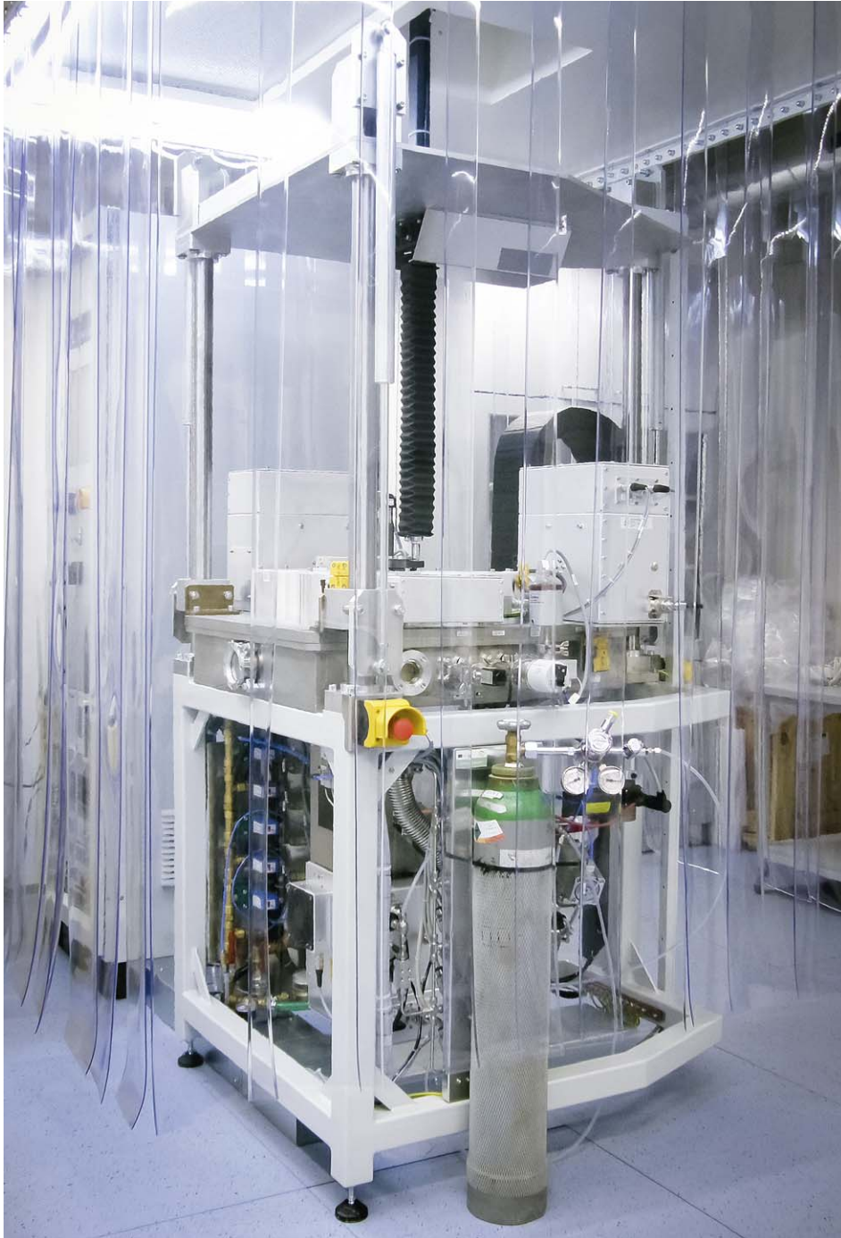
Computer controlled magnetron sputtering system Aurion
