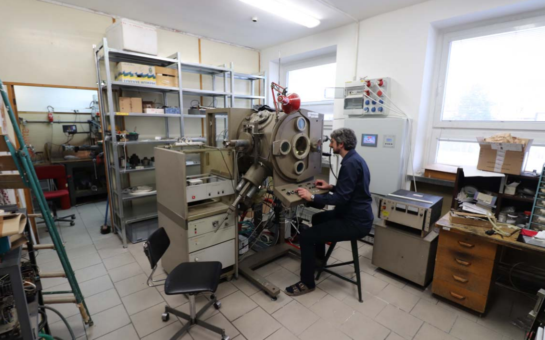
Electron beam welder
