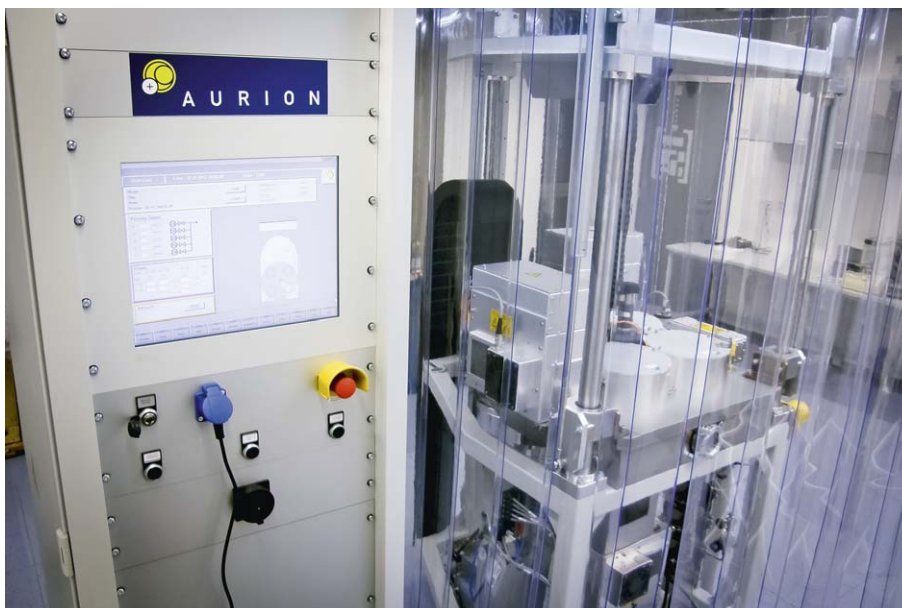
Computer controlled magnetron sputtering system Aurion
