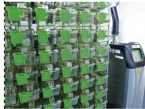
Rack for individually ventilated cages for accommodation of mice
