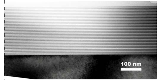
Cross section of the Si/C multilayer on silicon substrate
